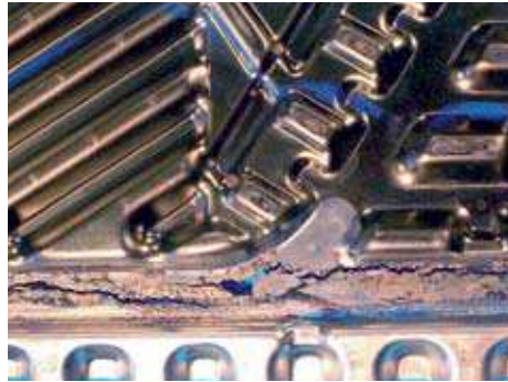
The wrong gaskets or poor gluing can cause leakage. The wrong glue may even destroy the plate.
