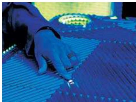
We search for pinholes and deformities with advanced techniques, including dye penetrants and UV illumination. This lets us find even the smallest crack.
