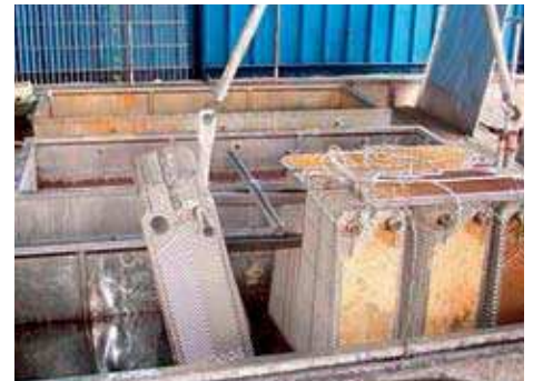
To ensure the perfect cleaning cycle, we rely on specially designed hydrojet cleaning or specialized chemical baths with the right concentration and temperature.
