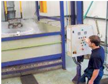
With media such as liquid nitrogen and caustic soda, we remove gaskets gently and completely, leaving the groove intact.
