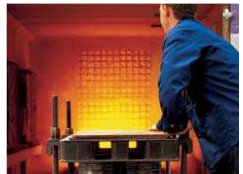
We use an oven-cured, two-component epoxy for PHEs that are frequently opened, so that gaskets stay in place after countless openings.
